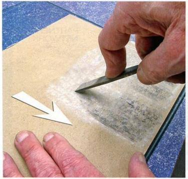
Finally, to enhance the chisel's cutting edge, we produce a slight "micro-bevel" on the beveled edge by stroking downward at a 45° angle approximately five times. This step enhances and extends the chisel's sharpness.
