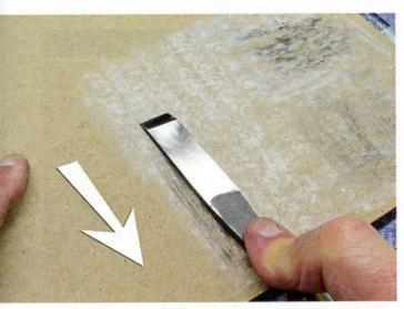
As in previous steps, the chisel is stroked on the flat side 15-20 times. The black discoloration is caused by particles of the metal being rubbed off the chisel.
