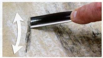
The technique for shaping, sharpening and honing gouges is similar to that for chisels. The only difference is that the gouge is stroked from side to side with a rocking motion; it still maintains that ever-important 22.5° bevel angle.
