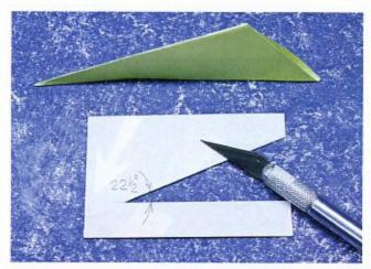
Using an X-Acto\* knife, cut out the 22.5\* angle and the template is ready to use.
