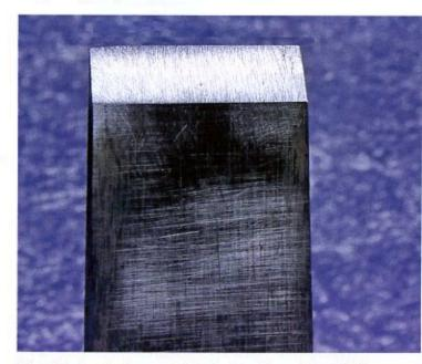
When the shaping is completed, the bevel face of the chisel will look like this, with rough striation milling marks. The subsequent refining steps will eventually produce a clean, smooth, mirror-finish bevel and a very sharp edge.
