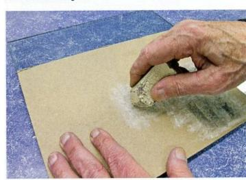
When the silicon-carbide steps are complete, the chisel is ready for the final step of honing. No leather strops are needed here; we simply rub a stick of white jeweler's rouge on a piece of cardboard.
