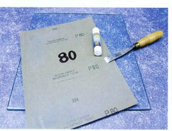
Use plate glass to ensure a true, flat surface. We begin with an 80-grit, silicon-carbide waterproof sheet that's glued to the glass with a glue stick.
