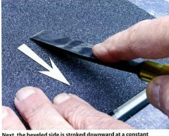
Next, the beveled side is stroked downward at a constant angle of 22.5° for 15-20 strokes. The burr that formed in the previous step will be eliminated, and a new burr will form on the beveled edge.
