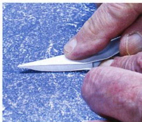
Fold the 45° angle in half to yield a 22.5° angle, which is close enough to 23°.
