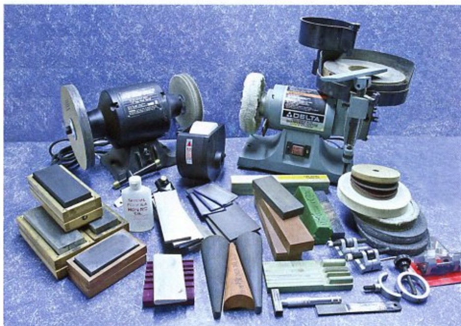
Here are tool-sharpening gadgets I've bought over the years in my quest to produce the finest sharpened chisels. Note the grinders, oil stones, wet stones, diamond stones, honing oil and various gadgets. All will be trashed soon – thanks to our new sharpening technique.
