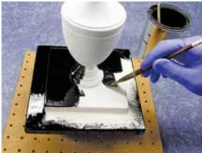
After the three primer coats, we apply two topcoats of high-gloss, bulletin-color, oil-based, enamel paint. Between these coats, we rough-up the surface with synthetic steel wool. This helps the second coat's adhesion, and improves its coverage.
