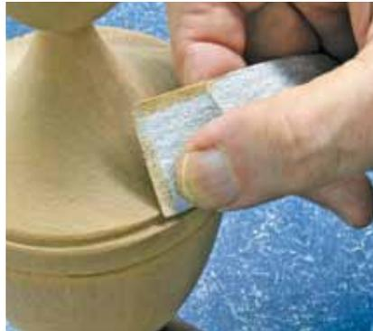
After sanding with the initial aggressive grit, we finish with finer, 120-grit abrasive.
