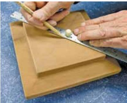
To permanently attach the finial to the cap, we first determine the cap's center by drawing intersecting diagonals.
