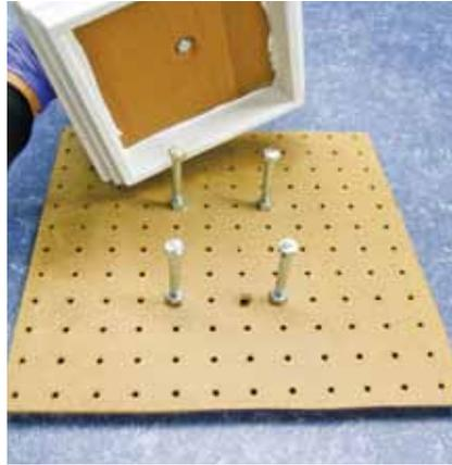
To allow the fin/cap to "float" during the coating process, we built a "bed of bolts" on a pegboard base.
