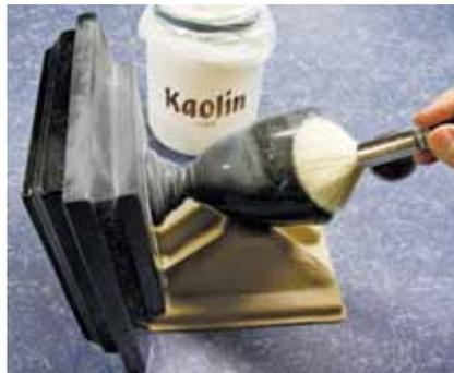
Dusting the finial and the upper portion of the cap with kaolin USP prevents goldleaf from adhering where it shouldn't (known as "shiners"). Also, it eliminates the need to contaminate the size with pigment.
