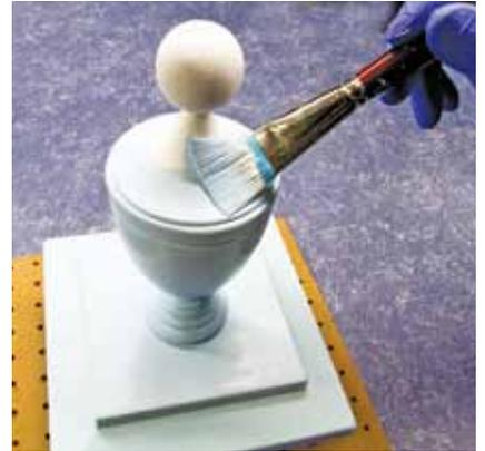
A light sanding with 220-grit sandpaper after the first primer coat removes any raised wood grain. We tint the second coat to ensure complete coverage.
