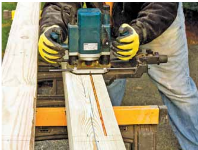
With a handheld plunge router, equipped with a side gate and a V-shaped bit, we run the first outer flute.
