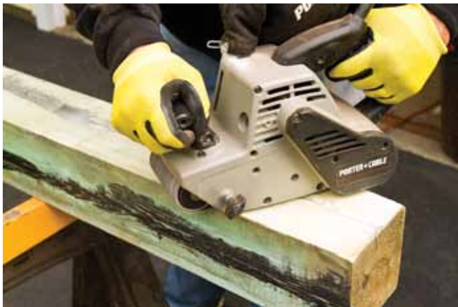
With the aid of a heavy-duty belt sander, we clean up the silicone patchwork first with a 60-grit belt, which we follow with 120 grit. On the first pass, we run across the grain to smooth the surface rapidly. Subsequent passes follow the grain.
