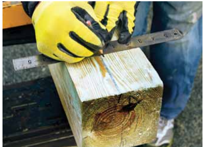
After the caulking and sanding are complete, we start marking down measurement guidelines. With the aid of a "centering ruler", we establish the center of the post.
