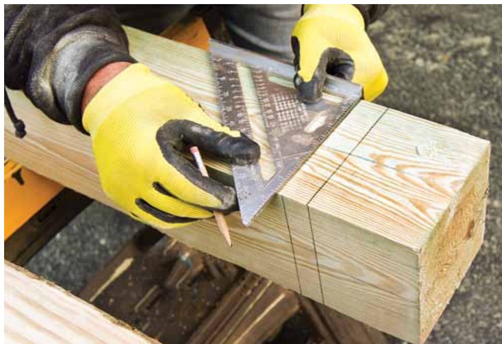
We place two lines, one 4 in. from the top of the post and the other 1 in. below that. Our central-flute line will start at the 4-in. mark and end at the pre-determined length of the substrate panel. The two side flutes will start at the 5-in. line.
