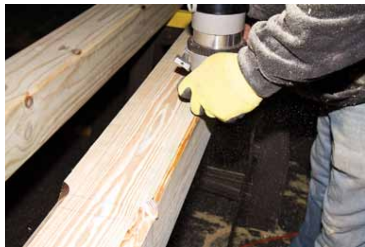
The last routing step is to use a large bit to round over all 90° edges that haven't been chamfered.
