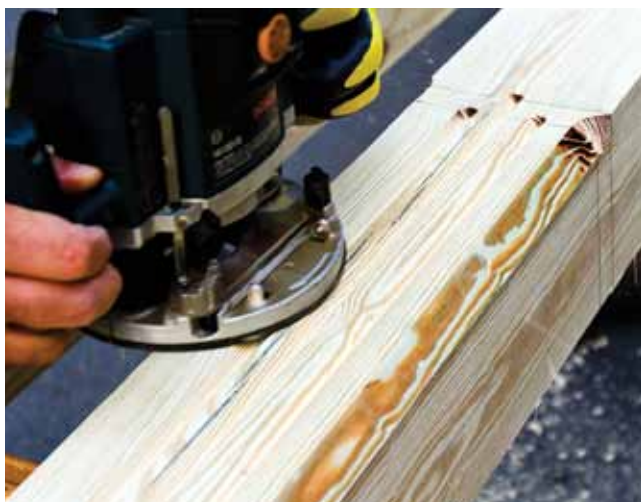
After the three flutes are cut, we use a large chamfering bit to place a chamfer cut, which equals the length of the central flute.
