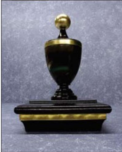
This finial and cap illustrates three gilded surfaces: spherical at the top, curved at the upper band, and flat on the bottom stripe. The latter is etched to help light interact with the gold. The other two curved surfaces need not be etched because light naturally interacts with their gilded curved surfaces.
