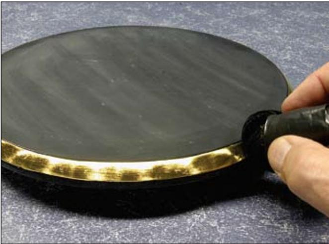
The simplest etching technique on gold leaf is "engine turning." It is accomplished by rotating a rounded piece of velvet cloth on the freshly applied gold.
