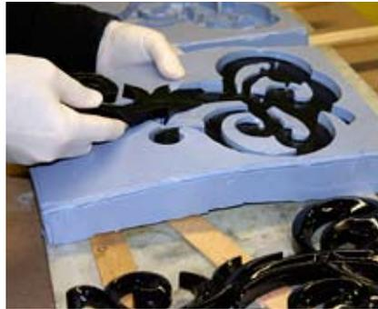
oil-based, Ronan bulletin paint. After forming a liquid-silicone mold around the original, he poured in liquid-polyurethane resin, which formed a replica scrolls after 10 minutes of curing.
