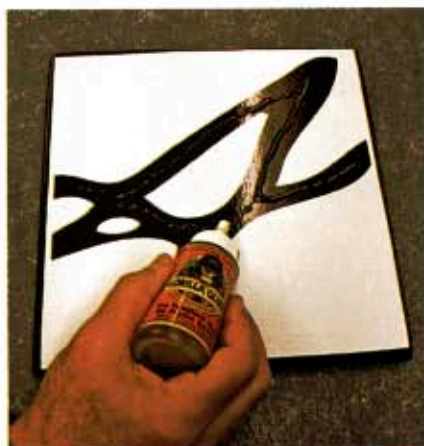
After covering the panel's undecorated portion with Gerber's removable-vinyl mask, cover the exposed area liberally with Gorilla Glue® adhesive.
