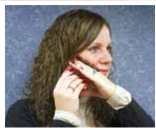
Photo 20: Each side of the gilder's tip may be "charged" with a small amount of facial oil by holding the tip against the cheek with one hand and pulling down with the other. (Jewelry is optional).
