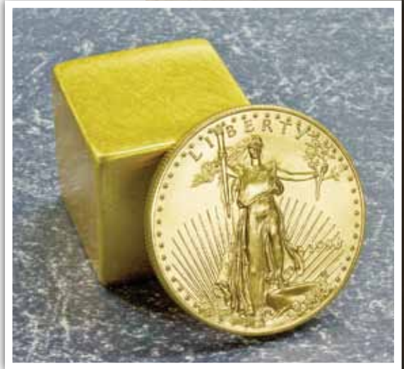
Photo 1: One ounce of U.S. gold currency coin worth about $1,680. The "gold" 1" cube is actually gilded Plexiglas. If pure gold, it would weigh 11.3-oz. And be worth more than $18,000.
