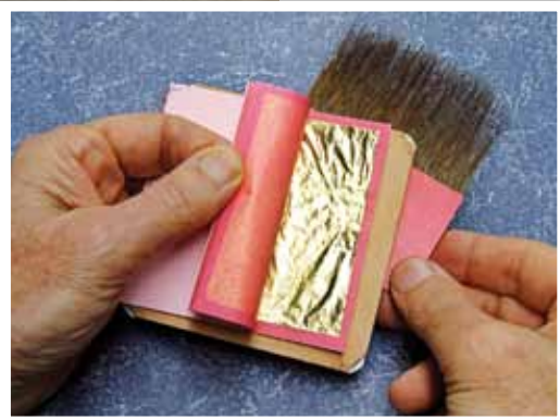
Photo 22: To momentarily store the gilder's tip while cutting the gold leaf, place the tip behind the booklet.
