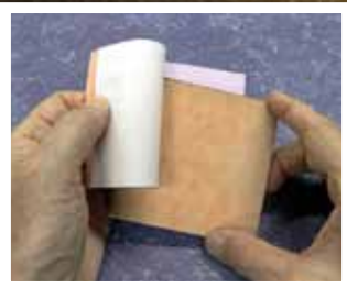
Photo 16: By inserting a leather square backed by a thin metal square, the booklet is rendered rigid for cutting purposes.
