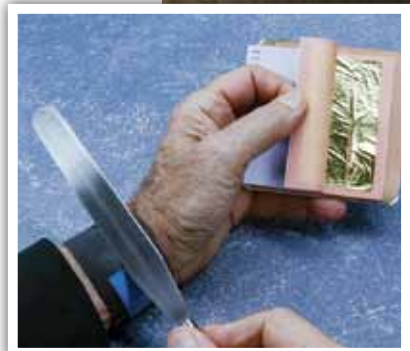
Photo 18: If gilder's knife snags the gold leaf, the knife can be honed on a 600-grit band conveniently taped to wrist.
