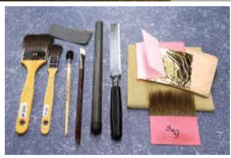
Photo 14: Loose leaf gilding tools: (l. to r.) Large gilder's "tamping" brush, small gilder's brush, pointed gilder's brush, white sable brush, 600-grit sand paper (above brushes), ceramic honing rod, gilder's knife, booklet of 25 sheets of loose gold leaf on a gilder's pad, and gilder's tip.
