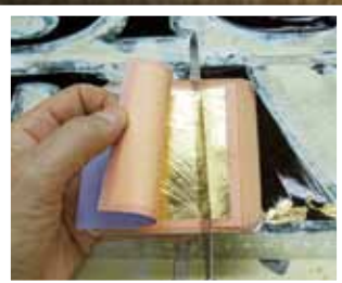
Photo 30: Covering cured size with just the right amount of gold leaf is almost a geometry problem. It requires judgment, assessment, and anticipation in how much gold leaf to cut.
