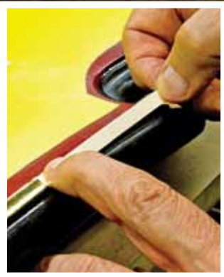
Photo 13: Patent strips are applied to sized cove by pressing gently on the backing sheet. Cutting strip with minimal overlap preclude wasting gold.
