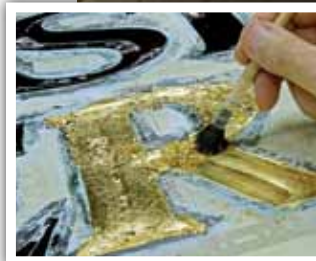
Photo 32: After completing the gilding of each letter, it is de-skewed to prevent skewings from spreading.
