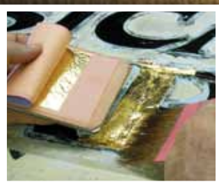
Photo 31: When gilding several lines of text, work from the bottom to the top to avoid contacting the cured ungilded size.
