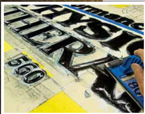
Photo 5: Before sizing, the overlap paint is sanded down with 80-grit sand paper to insure a clean, crisp edge on carved text.
