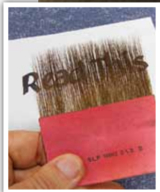
Photo 19: Thinning the hairs of the gilder's tip facilitates visibility through the tip while gilding.
