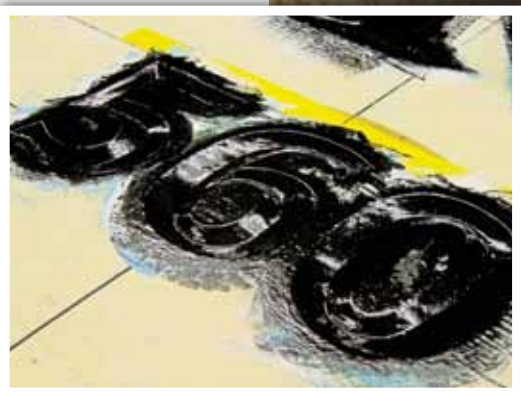
Photo 4: After carving through a pattern and removable yellow vinyl mask, text is primed and top coated with black enamel bulletin paint.
