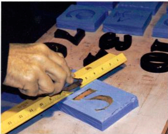
Lestingi measures and cuts a casting mold with a box-cutting knife.
