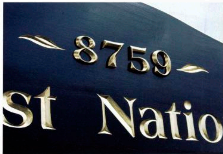
Cast-resin items interact well with size and goldleaf — they resemble handcarved items when installed.
