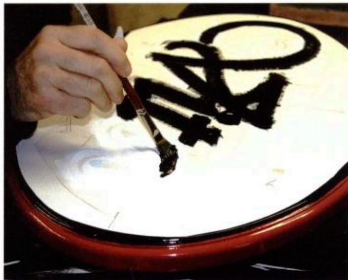
Three coats of Jay Cooke's sign primer and two coats of T.J. Ronan bulletin enamels, applied with a lettering brush, cover the face.
