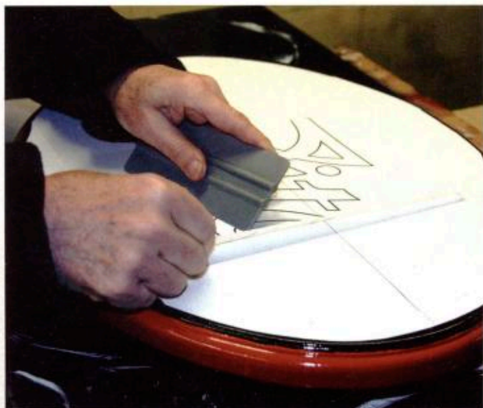
Lestingi applies the GerberMask II layout pattern with a squeegee.
