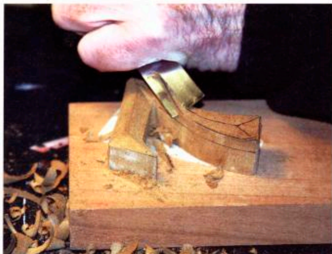
Using gouges and chisels, Lestingi fashions a numeral that he'll cast for future use.
