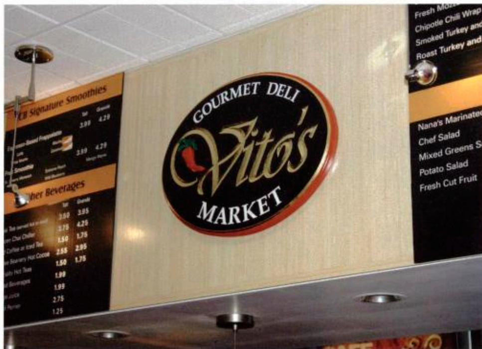
This sign comprises an Extira™ composite-material panel, cast letters, a border detailed with a bead-and-cove profile, and years of handpainting and gilding experience.
