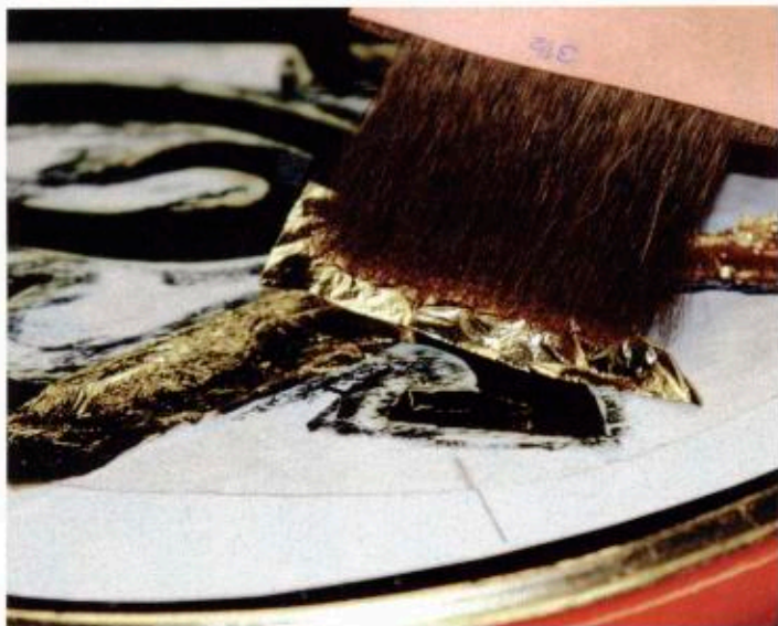
Lestingi applies 23k, surface leaf to the letters with a gilder's tip.
