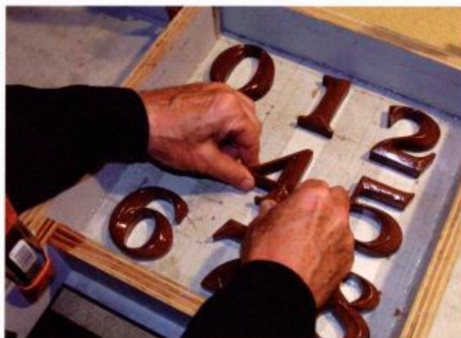
The carved numerals sit in the confinement field, awaiting a two-part, liquid-silicone, casting product that creates molds, which can be used for future projects.
