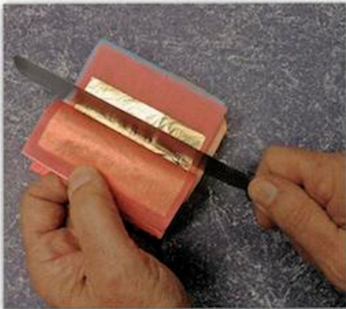
Since full sheets are not needed in most cases, a gilder's knife is used to cut the gold leaf into smaller segments.
