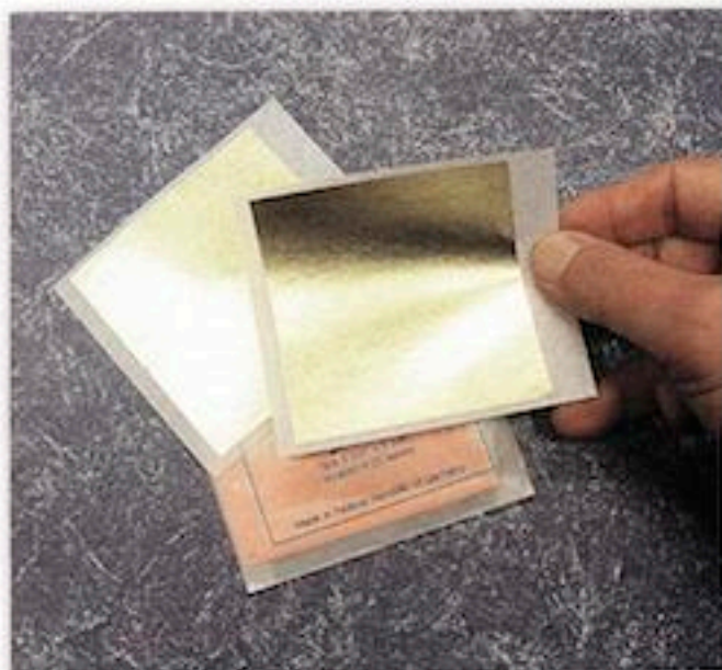
Lighter 'patent gold' may suffice when gilding cove borders, flat surfaces and other simple applications.
