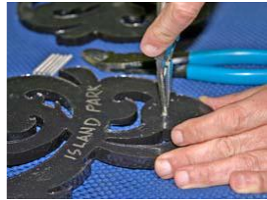
To attach the scrolls to the signface, he inserted 1/8-in., threaded-aluminum studs.
