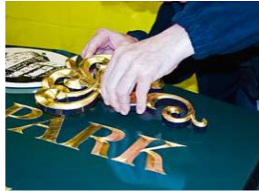
The filigree is nestled into pre-drilled, silicone-laden, signface holes.
