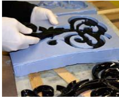
After forming a liquid-silicone mold around the original, he poured in liquid-polyurethane resin, which formed a replica scrolls after 10 minutes of curing.
