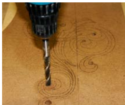
Lestingi cut the original filigree from Extira® wood-composite material. He used a scroll-blade saber saw and a drill to fashion them.
