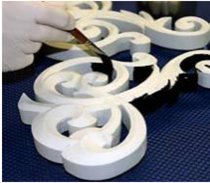
After priming the scrolls, he applied two coats of high-gloss, oil-based, bulletin enamels.
