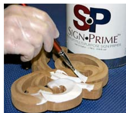
Before the casting process, he coated them with Sign Arts Products' Sign*Prime™ all-purpose primer.
