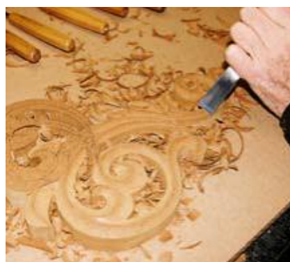
He carved the high-relief filigrees using a curved, sweep gouge and a straight chisel.
