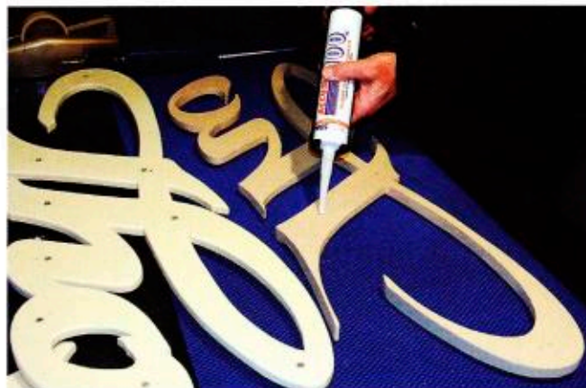
Using 6-in. deck screws and 100% silicone, he joined the separate layers of copy he crafted.
