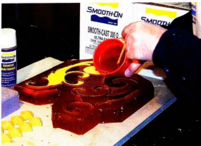
Francis molded accent scrolls using the Smooth-On (Easton, PA) casting system.
