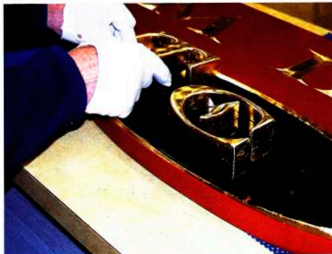
A shot of silicone affixed each letter of the logo onto the panel.
