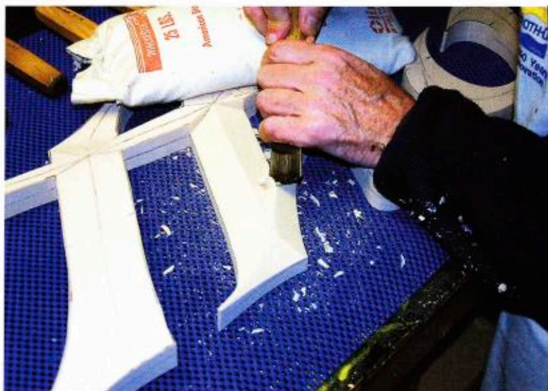
Francis anchored the letters using a 25-lb. bag of buckshot before he carved them.
