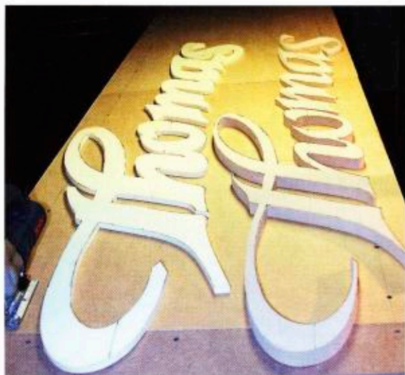
Using a saber saw, Francis cut the script from 1/2- and 3/8-in. HDU. He used the thinner piece as a frame and carved the thicker substrate to a high-profile, prismatic edge.
