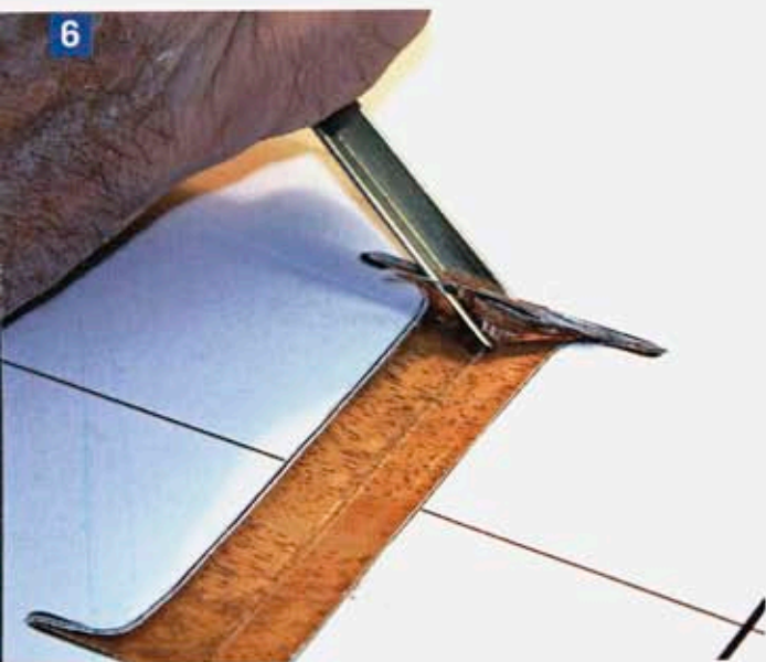
6 With the v-parting tool, re-establish the serif root lines.
