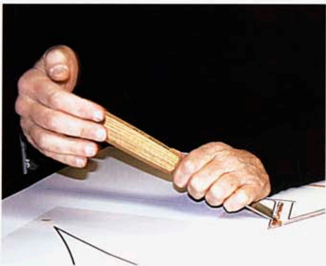
Some carvers use a mallet to push tool through the substrate, but I use my hand and a mallet pad between the palm and the tool.
