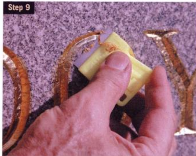
Step 9 After gilding, Francis cleaned up shellac and primer overlaps with a single-edge razor.
