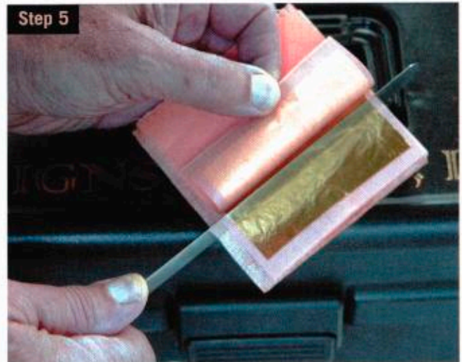
Step 5 Because he applied gold to small, incised areas, Francis cuts his goldleaf sheets in thirds with a gilder's knife.
