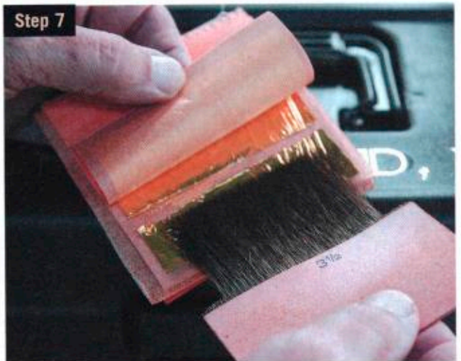
Step 7 Francis applied and oiled the tip to the book. The tip holds the leaf, but once he touches it to the sized areas, whose bond is stronger, the gold leaves the tip.
